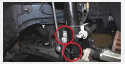
Remove the strut tower brace is applicable. Starting with either driver side or passenger side remove the wheel. Disconnect the brake line bracket and detach the ABS sensor wire from the strut body.
