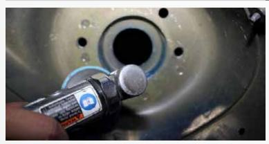
Check the bottom of the strut tower housing for any roughness. Use a Sander or sand paper to smooth out the Housing.
