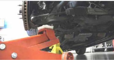
Support the lower control arm with a floor jack, remove the lower strut mounting bolts and lower the floor jack to remove the strut assembly.
