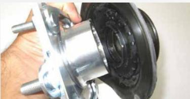
Install the Camber/Caster Assembly to the supplied Ford Strut Tower Pivot Assembly.
