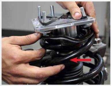
Place the Camber/Caster Assembly onto the Strut Assembly.
