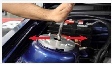
Center the strut shaft in the strut tower opening side to side. Once its center then tighten the 4 13mm nuts.
