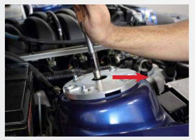
Loosen the 5 nuts on the Camber/Caster Plate assembly very slightly, until the plate can barely slide. Slide the entire assembly towards the front of the vehicle and tighten the 17mm Nut.
