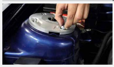
Re-install the strut assembly, place the cover over the strut tower where the studs protrude, don't fully tighten the top nuts. The factory strut tower brace can be used with this kit by placing the 2 ends above the decorative cover. NOTE! Remember to remove the rubber band holding the Camber/Caster Kit.
