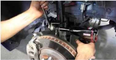
Remove the sway bar end link from the strut, then loosen but do not remove the strut mounting bolts.
