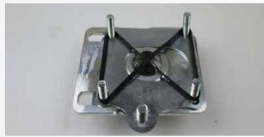
Place the Caster Plate on top of the bearing plate. Make sure that the raised lip around the bearing plate protrudes up through the center slot of the Caster Plate. NOTE! The use of a rubber band will help hold the stud plates in position while installing. Be sure the plates move from side to side smoothly.
