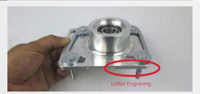
Determine which Camber/Caster Plate is driver or passenger side by looking at the engraved SUB768D for Driver side and SUB768P for Passenger side. Install the 2 provided stud plates from the bearing plate, with the studs protruding through the slots. NOTE! Make sure the larger radius between the 2 studs of each plate face the bearing.
